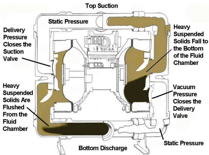
Slurry Valve pumps have a bottom discharge allowing the gravity assisted and free transfer of suspended solids through the pump. The top suction allows suspended solids to fall into the lower section of the fluid chamber. First the solids, then the fluid, is forced from the chamber through the discharge valve. Each stroke flushes the slurry solids using the fluid from the upper portion of the chamber.
