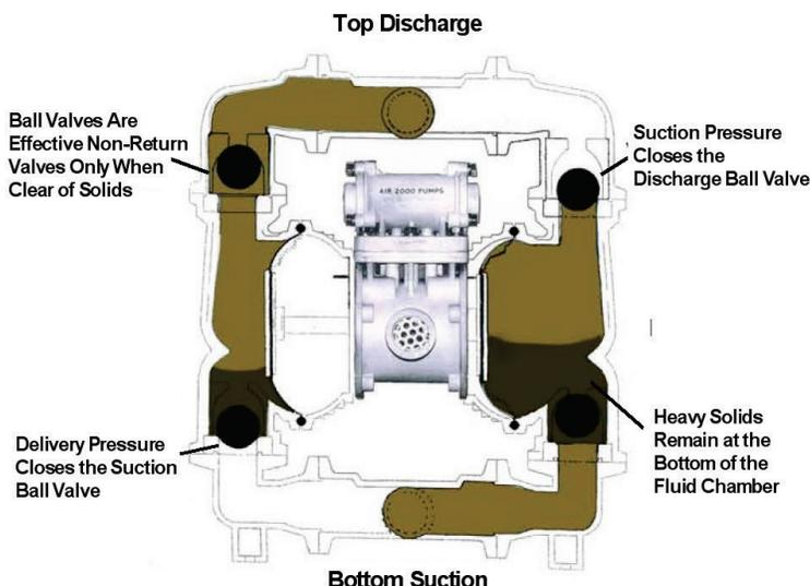
The ball valve seats horizontally allowing small solids to lodge between the cage, ball and seat. When a ball valve pump fails to seal it's valves, the pump
