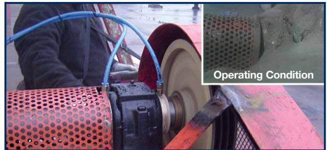
LabTecta-OAP-PB™ installed on a Pillow Block duty
